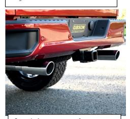
6. With proper clearance from spare tire, install the exhaust tip onto the tailpipe. The system was designed to have the tip 1" below the quarter panel of the vehicle. Note you can adjust the tip position inward or outward with rotation of the exit pipes.
